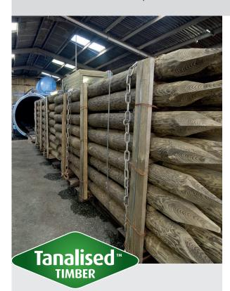
TANALISED timber is timber which has been impregnated with TANALITH wood preservative under rigidly controlled conditions in a vacuum pressure timber impregnation plant.
